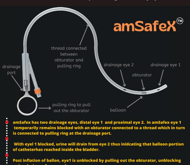
amSafex has two drainage eyes, distal eye 1 and proximal eye 2. In amSafex eye 1 temporarily remains blocked with an obturator connected to a thread which in turn is connected to pulling ring at the drainage port.
